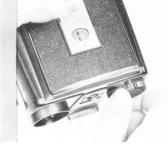
4 Break the film seal; then draw the paper, colored side out, over the side of the film holder marked FILM THIS SIDE. Thread the end of the paper fully into the longer slot of the empty spool. Turn the winding knob two full turns to make sure the paper is straight and tight. To make sure the paper is tight,
